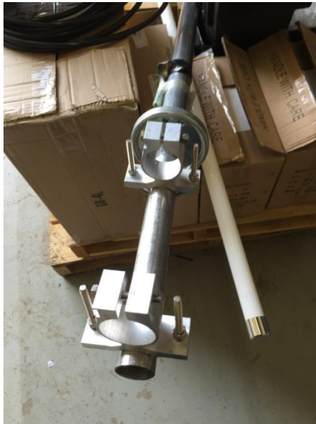
Figure 1 - Attach Antenna to the Mast
